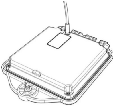
Figure 4.13 Charging the transmitter Li-Ion battery pack
