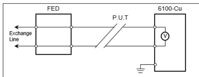
2. For **Open**, connect the T-R/A-B and ground wires to the customer side of the FED (blue labeled connectors).
